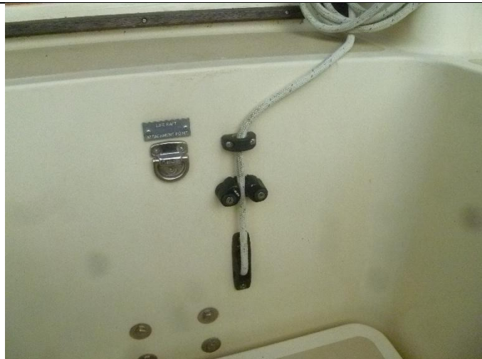
Simple centreplate lifting arrangements.
