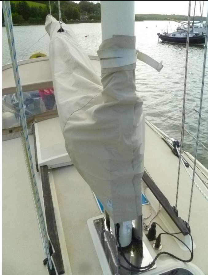
Mast, stepped in substantial stainless steel tabanacle.
